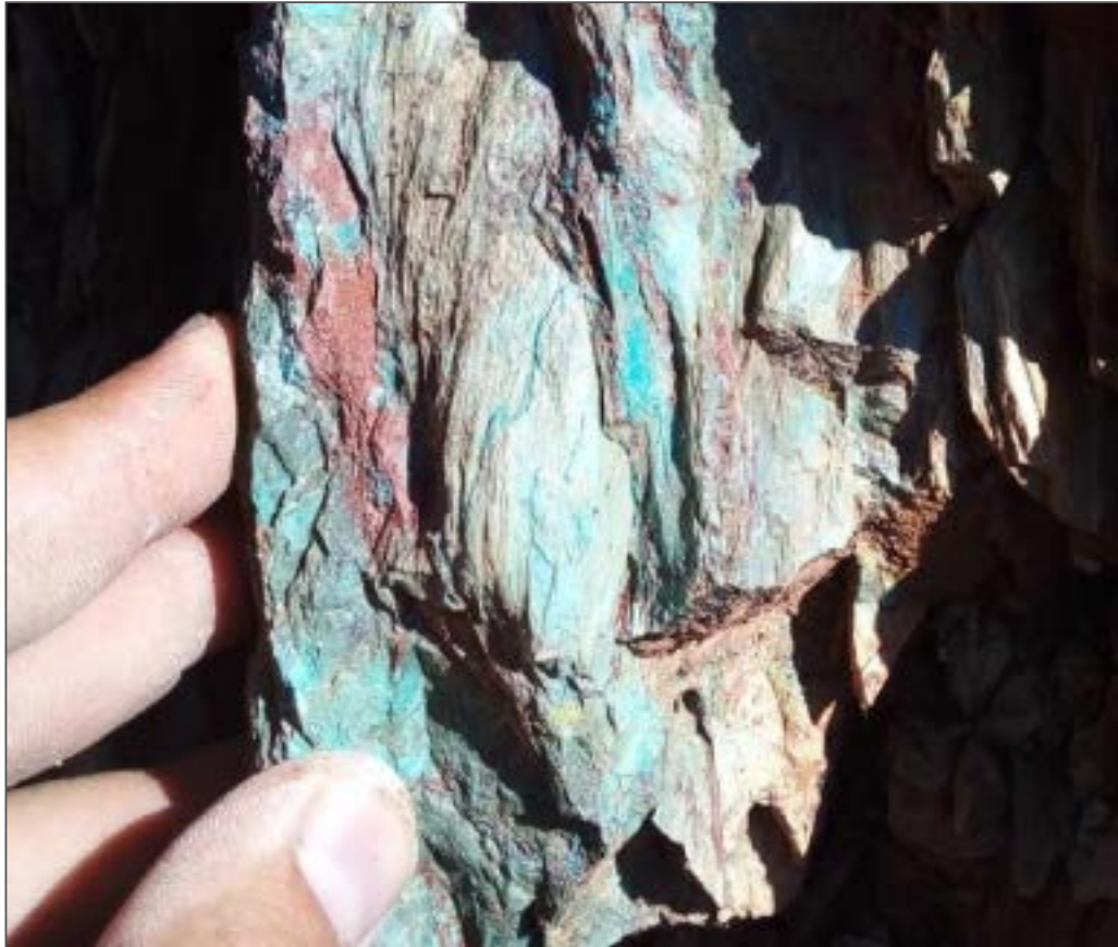
Figure 3-11: Copper mineralisation as found along the contact zone between the Otavi and Nosib Groups.
